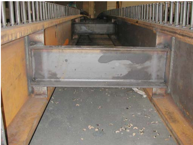
Fig. 17: Execution of detail of welded U-cross-beam connection to stiffening plates including web reinforcement of the main girder; left: practical example of fabrication; right: execution with drainage openings for galvanising
