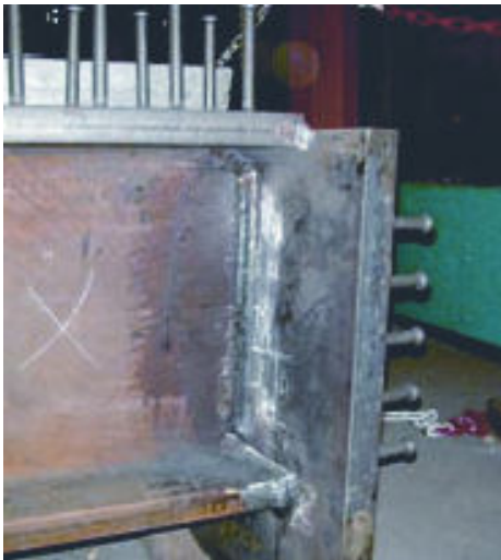
Fig. 12: Detail with welded-on end plate
